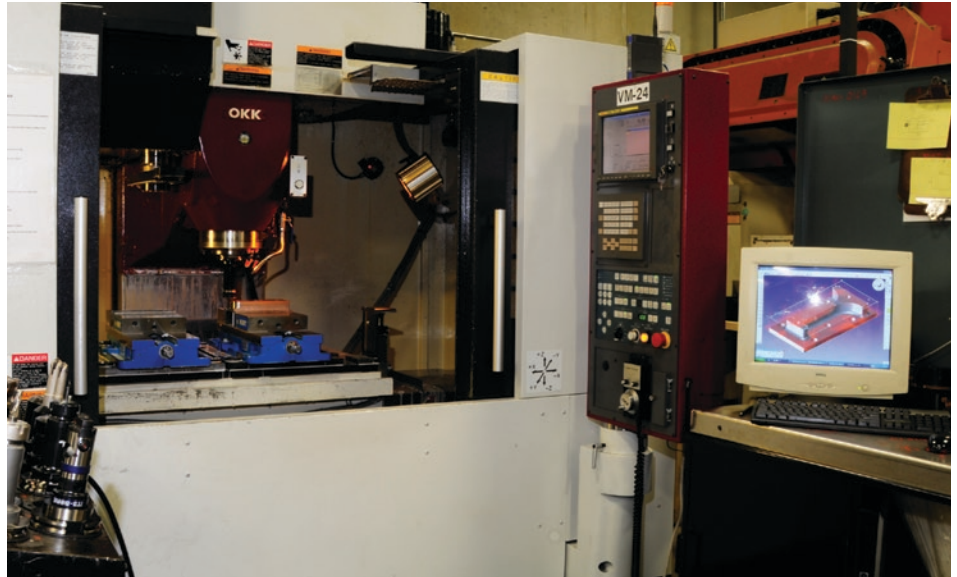
OKK MCV1060 CAT50 13K spindle machine.
