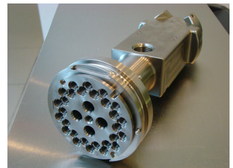
This Titanium energy industry component took 18 minutes to rough using a traditional toolpath and only 11 minutes using a VoluMill™ toolpath.
